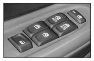
The controls for the power windows are located on the armrest on each of the side doors. With power windows, the switches operate the windows when the ignition is in RUN, ACCESSORY or when Retained Accessory Power (RAP) is active. See "Retained Accessory Power (RAP)" under *Ignition Positions on page 2-20*. The driver's door has a switch for each of the passenger's windows as well.
